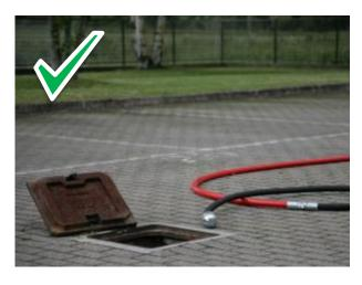
The ECOLEADER Sewer Leader Hose is a section of hose to be attached to the front of the main jetting hose.
