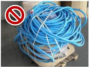
The first image represents some hoses well stored. These hoses are coiled onto a wooden bobbin or neat coil, protected from dust and environmental factors with protective packaging. The second image shows a improper storage. This hose could be severely damaged and also could be a danger for people that work close to the hose.
