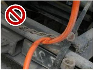
Effects of twisting a hose. This stress could severely damage the hose.
