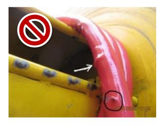
Unsuitable hose drum could squash and damage the hose during application. The white arrow and the black circle underline the effect of this improper use.
